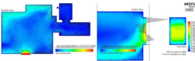
Simulation (figure 5) provided insight into actual flow efficiency coefficient for calculating air change rate based on east wind vector component perpendicular to facade opening (Swami, Chandra, 1987):
