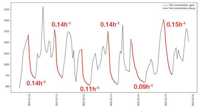
As shown in figure 3, dormant hours time period, with low average air change rate due to highly sealed facade openings, is insufficient to provide enough fresh air with natural infiltration concentration decay, so stale and polluted air is building up as time progresses. This issue is accentuated during winter months when outdoor air pollution in Sarajevo area is usually high (IQAir, n.d.).
