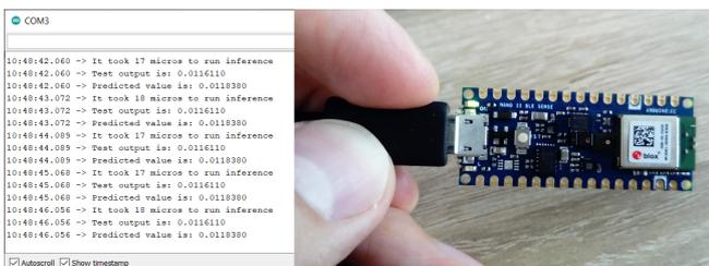
Proposed algorithm concept (figure 8) for microcontroller uses TinyML neural network to forecast absolute humidity
