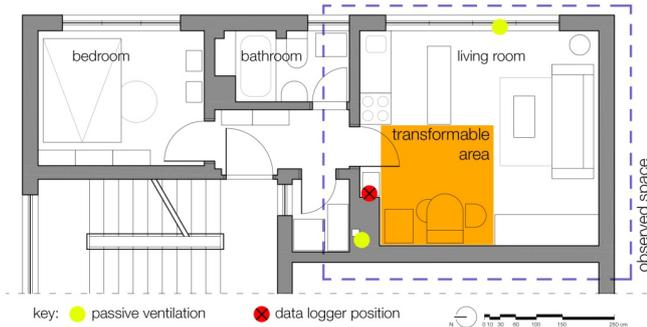
Data was collected during months of winter 2020/2021 season. Data logger (Avdić, 2020) was built upon Croduino Nova (ESP32) microcontroller with SGP30 air quality sensor, SHT20 temperature/relative humidity sensor and analog optical dust PM2.5 sensor programmed in Micropython (figure 2a). Sensor data was written in 15 minute intervals on microSD card, including web data from local weather and air quality stations. In preprocessing phase, data was cleaned up and merged to hourly logs (figure 2b).
