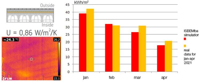
This confirmed average U-value of 1.14 W/m<sup>2</sup>K for apartment enclosure (Arnautović – Aksić et al., 2016) in observed space, along with critical thermal bridges in facade walls for dew point calculation. Based on U-value and temperature difference we can determine interior surface temperature ( $T_w$ ) for recognized critical points (Hadrović, 2010):
